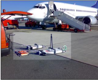
With SeCon, the nondestructive sensory Control system we measure the quality of paved fields by ground radar from the surface over the bound base to the unbound layer.
